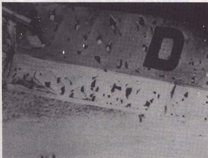
A section of D-12-348's wing after it had been returned to the Wasserkuppe. Damage is from hail.
