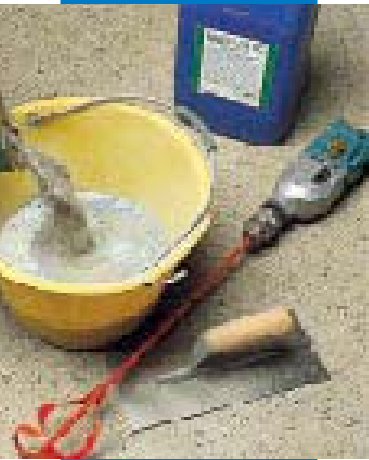
Mixing of Mapelastic with a mechanical mixer
