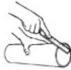
Chamfer end of pipe, using medium file or rasp. Standard lengths of pipe are already chamfered
