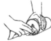
Remove swarf, dust and file dirt from end of pipe
