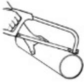
Cut pipe square, using fine tooth saw. Wrap paper around pipe as guide line
