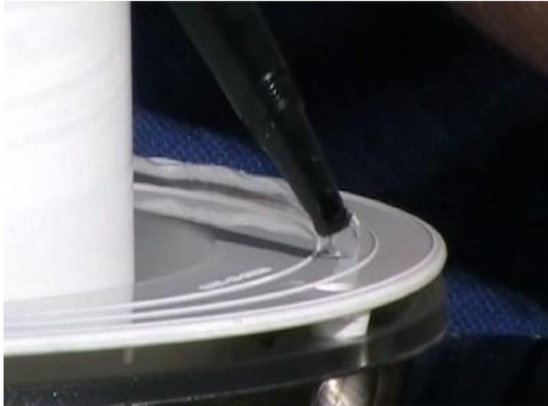
11. The Stixall should be applied in one continuous bead and joined onto itself. There should be no breaks within the bead.
