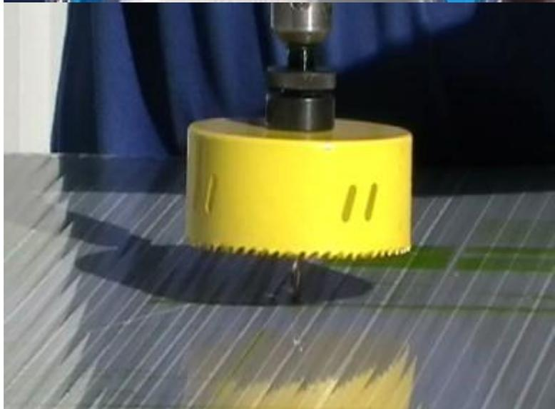
7. Cut the hole in the sheet, ensure that any rough edges are smoothed and that any debris that has entered the sheet is removed. This can be done with either an air compressor, a good vacuum or the debris can be washed through but the sheet will then need to be left to dry out.
