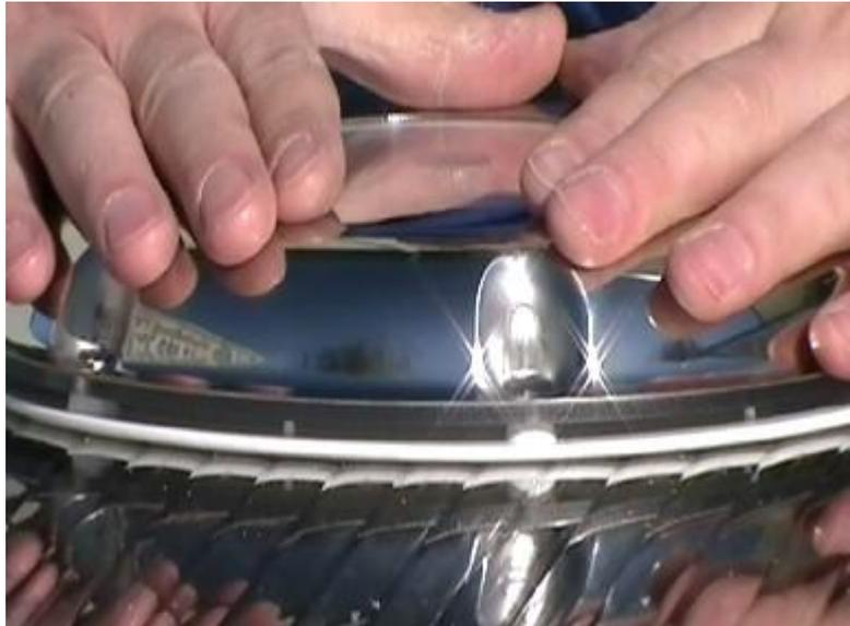
14. Leave the vent undisturbed in the sheet for a couple of hours to allow the adhesive to set before continuing.
