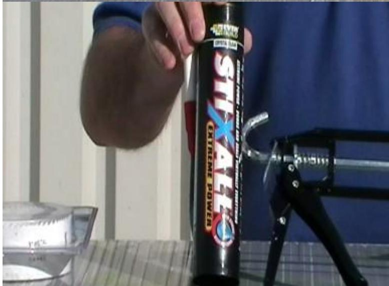
10. The Stixall should be applied with a generous bead, ensuring that the Stixall remains within the tramlines.
