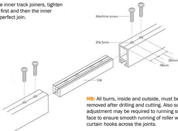
**NB:** All burrs, inside and outside, must be removed after drilling and cutting. Also some adjustment may be required to running surface to ensure smooth running of roller wheel curtain hooks across the joints.
