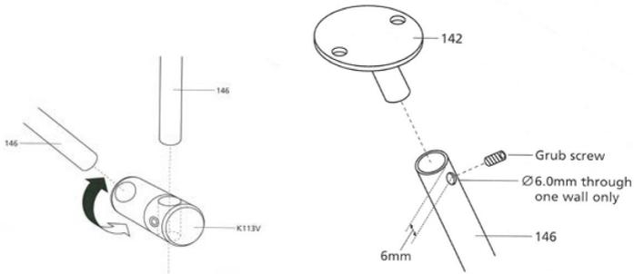
**10.** For V-suspension, please refer to Fig.2. When assembling the 313 hanger assembly, ensure that the K113 V-hanger is located on the suspension tube and is resting on the lower 113 hanger which is fixed to the track.
