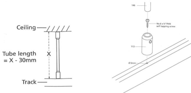
**9.** At no point should the track span more than 3000mm without support. If the track has a join, ensure the track is suspended within 150mm from the join. If the track has no lateral support and spans more than 3000mm, please ensure a V-hanger is used. Using a plumb line mark where the hanger assembly will fix to the ceiling and track. Refer for Fig. 2
