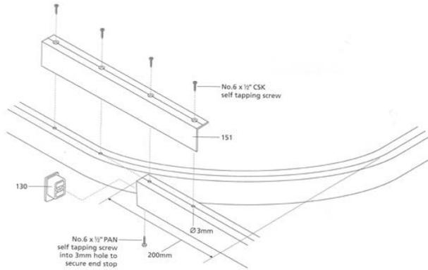
8. For suspension rods refer to Fig. 1. Each bend must be supported by a 313 hanger assembly no further than 350mm from either leg of the bend.
