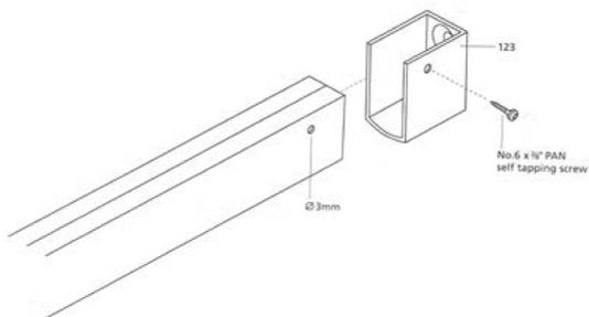
7. Depending on layout of the track, join each section together with overlaps, taking care that all fixing holes are used and screws are tightened securely for maximum stability.
