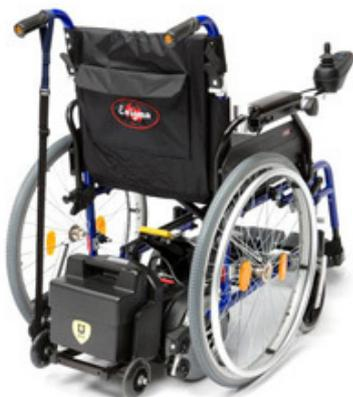
Designed as an electronic wheelchair, with a user-controlled powerstroll the user takes charge of the chair's direction and speed through the use of a joystick.
