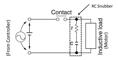
Drawing below shows how RC Snubbers could be implemented near the shade motor in a junction box.
