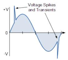
The high voltage spike coming back down the power cable through the blind controller (generally just a relay) reaching back to the Circuit breaker is what causes it to trip.
