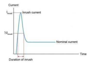
A good LED driver or switch mode power supply will have built-in current limiting eradicating the problem of passing the inrush current down the chain to the circuit breakers. Beware of non-branded or cheap imported units, do a bit of homework before purchasing.
