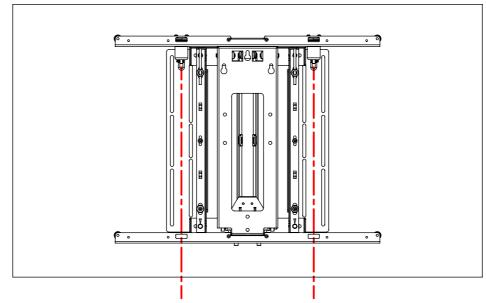
No Cable Routing Bosses used Cables hang below the screen
