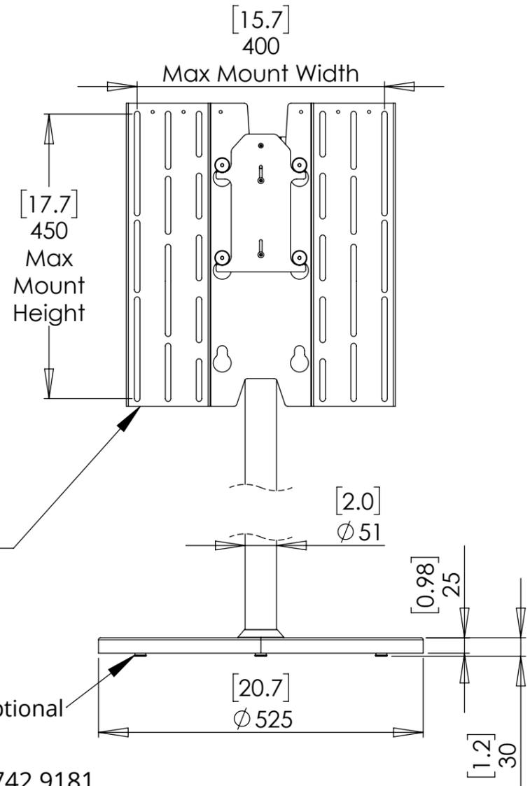
Quick release mount can accommodate bolt patterns up to VESA 400x400.
