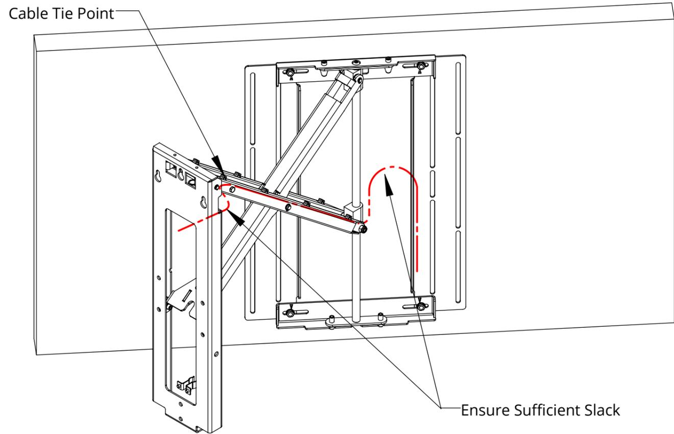
Wall sockets should be ideally placed as shown outside of the bracket footprint to maximise space for cable routing
