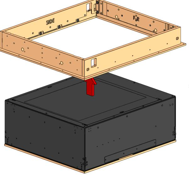
For quick and simple install, mechanism easily clicks into supplied pre-install framework.
