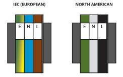
The Power supply is compatible with world-wide mains voltages and Frequency. e.g., UK 240V 50Hz and USA 120V 60Hz. The power feed should be from a protected (fuse or circuit breaker) line. Fuse or Circuit breaker rating should be adequate to protect the cable type and size used to supply the SPU10 in the event of wiring fault.
