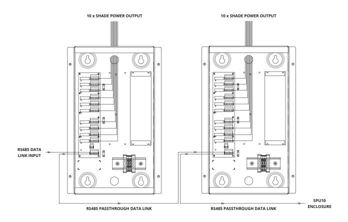
To daisy chain the RS485 signal between multiple SPU10 units, the RS485 source from the control system will need to be wired to the "RS485 Input / Data Link" connector on the first SPU10 panel. A second cable can then be bi-wired out of this "RS485 Input / Data Link" connector into the "RS485 Input / Data Link" connector in the next SPU10 panel along in the chain. The maximum number of SPU10 panels than can be daisy chained together will vary depending on individual panel loading.
