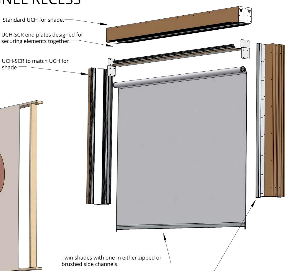
Side Channels mounted inside UCH-SCR and covered by removable flap supplied
