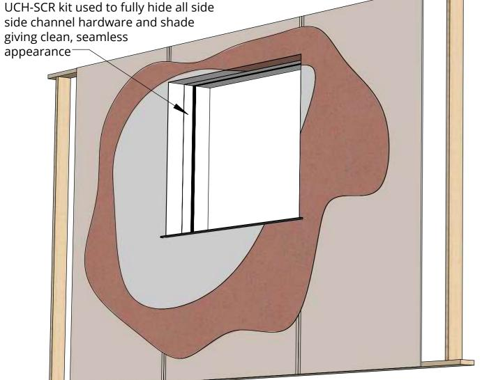
Standard UCH for shade. UCH-SCR end plates designed for securing elements together. UCH-SCR to match UCH for shade
