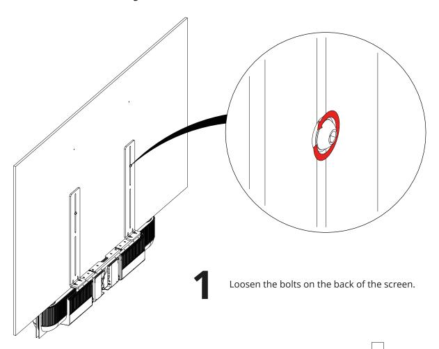
Adjust the height of the speaker. Once in position, retighten the bolts.
