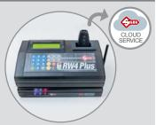
Original key reading. Data are sent via cloud to Silca for processing.
