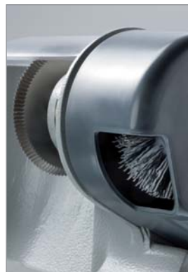
Incorporated brush for finishing cut keys
