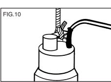
If pumping water from a sandy or muddy floor bed, the pump can be suspended using a rope or chain (not supplied) fixed to the handle. DO NOT use any of the electrical cables for this purpose.
