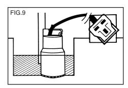
When submersing or lifting the pump it will be necessary to use a rope or chain, this must be attached to the transport handle.
