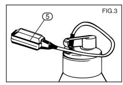
As the water level drops the float switch will fall with the water level.
