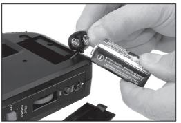
The detector is powered by a 9V PP3 type battery.
