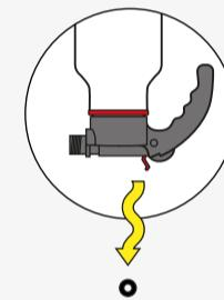
Remove the top of the mechanism. Pay attention that O-ring **A** (1,78 x 1,78 mm) comes along. If not, shake it out by holding the pump upside down.
