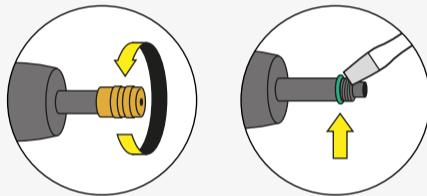
**2** To get inside the pump sprayer's mechanism, you will need to unscrew the spray head first.
