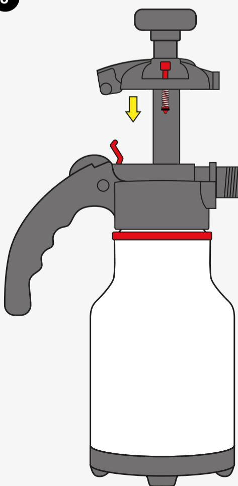
Click the top back onto the bottom of the mechanism. Make sure that the O-ring **A** (1,78 x 1,78 mm) remains in place. Finally, screw the spray head back onto the mechanism.
