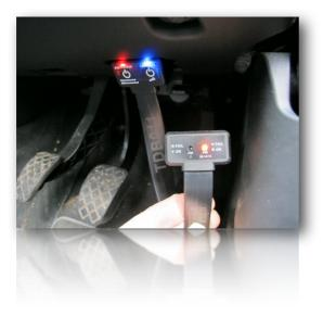
CHECK THE POWER IS CORRECT AND THAT PIN 7 IS <u>NOT</u> ILLUMINATED.
