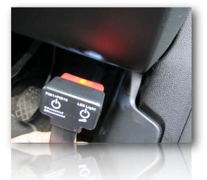
TOUCH THE IGNITION BYPASS SWITCH AND THE RED LED WILL ILLUMINATE.
