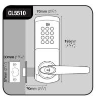
Outside handle and key functions as before. Lock case key will double-throw the deadbolt, retract the deadbolt and retract the latchbolt without the code. When deadbolt is thrown it denies access by code. The anti-panic feature allows the inside handle to simultaneously retract the latchbolt and the deadbolt preventing people being accidentally locked in.
