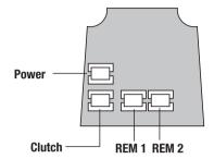
**REM 1** is for connection to a reception desk push button or a door intercom system. Pressing the button will cause the keypad to flash blue on the lock and release the lock for the pre-set time.
