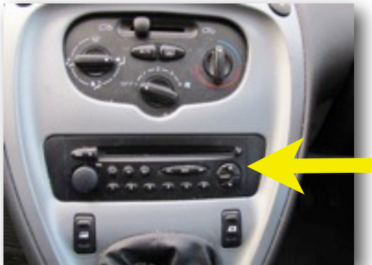
VEHICLE DOES NOT HAVE CAN BUS DIRECT ECU CONNECTION REQUIRED
