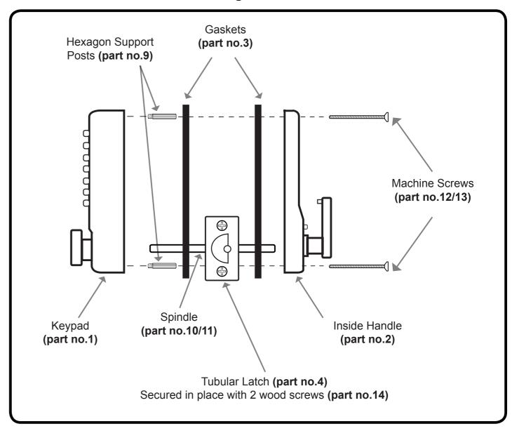
Place the remaining rubber gasket (part no. 3) around the back of the inside handle and as with the keypad side the spindle follower on the back of the inside handle will need to be visible.
