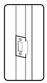
Push the door to the closed position and mark the area on the frame of the door where the strike plate would need to be fitted.
