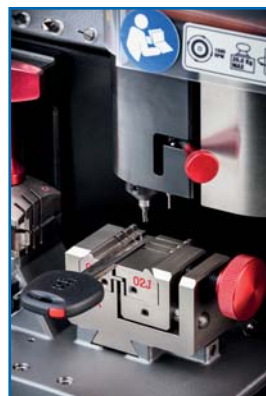
Laser and dimple key cutting station
