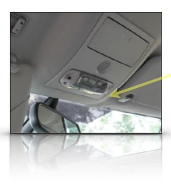
LOCATE THE RF MODULE WITHIN THE VEHICLE
