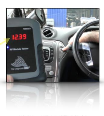
TEST 1 : PRESS THE START BUTTON AND THE TDB023 WILL SOUND AND FLASH WHEN THE SIGNAL IS RECEIVED
