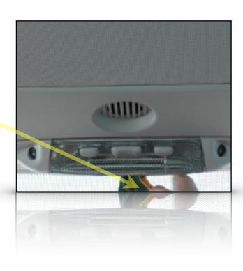
USING A TRIM REMOVAL TOOL, GENTLY EASE THE PANEL FROM IT'S POSITION
