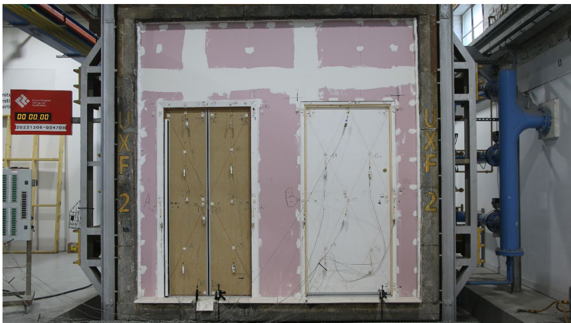
Figure 17 - The unexposed surface of the test construction prior to the commencement of the test
