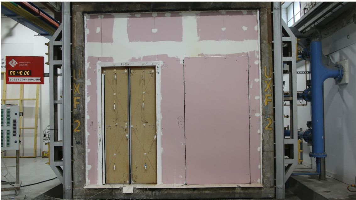
Figure 21 - The unexposed surface of the test construction after a test duration of 40 minutes
