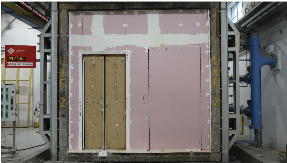
Figure 22 - The unexposed surface of the test construction after a test duration of 50 minutes
