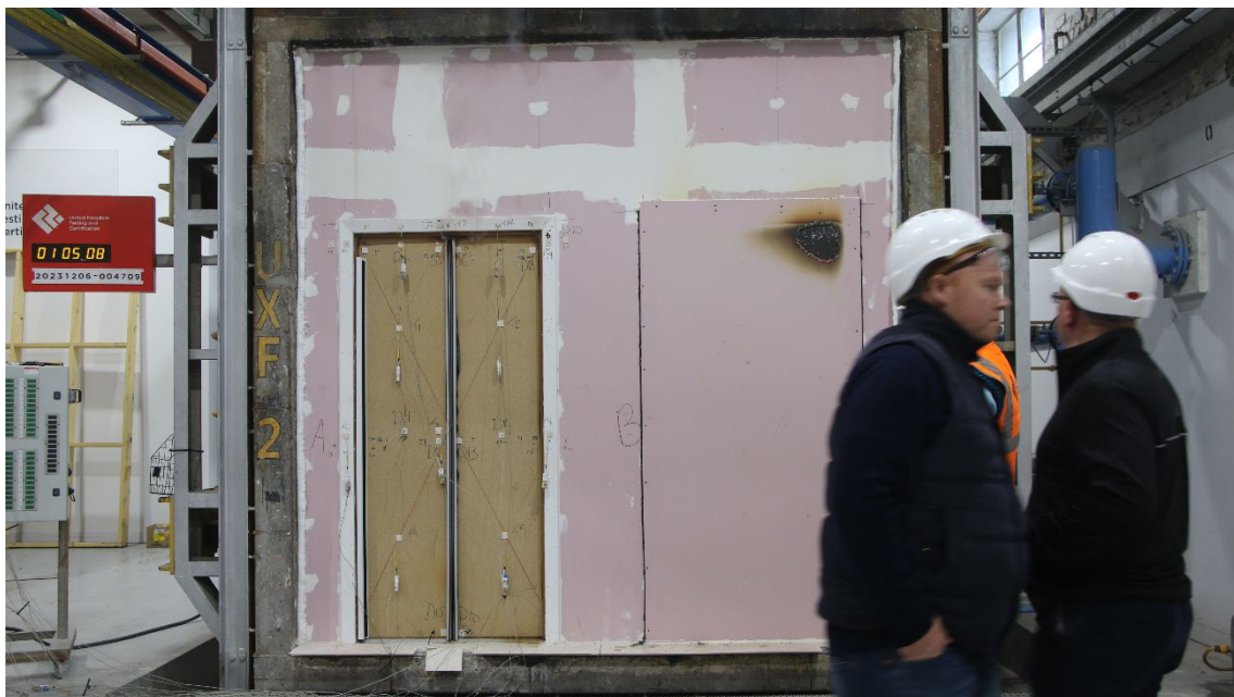
Figure 25 - The unexposed surface of the test construction after a test duration of 65 minutes
