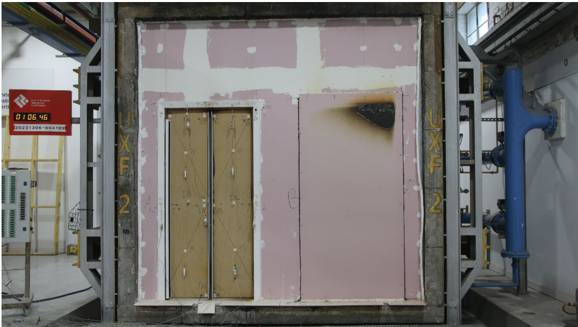
Figure 26 - The unexposed surface of the test construction after a test duration of 66 minutes
