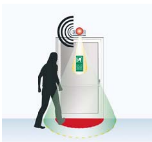
Prealarm 2: visual/audible alarm with additional light spot
