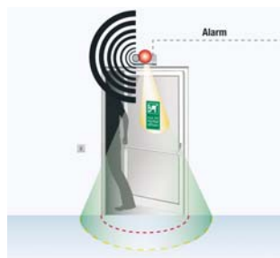
At door opening: main alarm is transmitted to control centre (optional)
