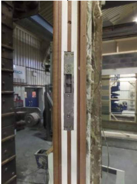
Top latch forend in frame head – doorset B
