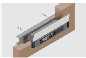
The Letterbox key safe can be installed directly into most existing letterbox flap/plate openings and is secured with a rear clamping bracket. If the existing letterbox flap/plate opening is not suitable there is a replacement face plate/flap. The LBX-KS comes with a built in retractable lanyard so the keys stay with the unit and not with the user.
