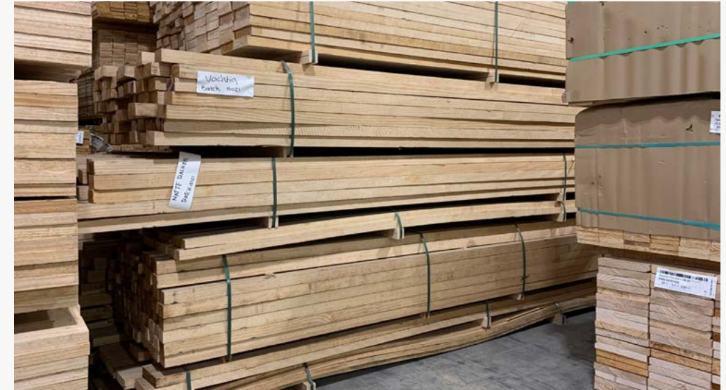
Bundles stored on top of each other; bearers aligned
