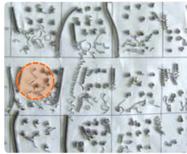
Competitor A • Thin and long chips are coiled around the holder.
