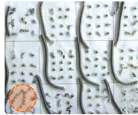
Competitor B • Folded chips under certain cutting condition • Poor chip evacuation
