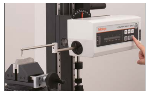
Centralised front control panel.
