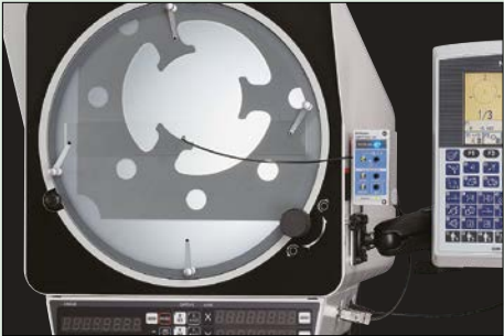
Locating the edge of a hole.
