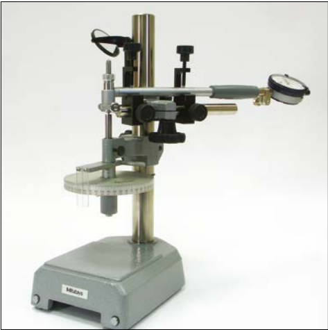
Calibrating a bore gauge.
