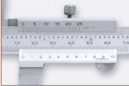
Decimal and fractional graduated scales (inch/metric models only).
