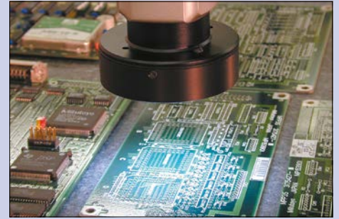
QVP probe inspecting a PCB.
