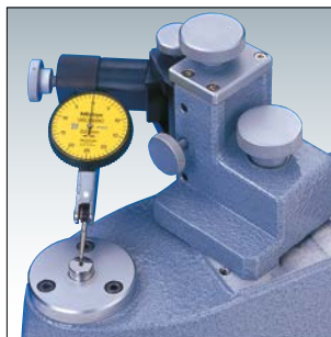
Calibrating a lever indicator (dial test indicator).
