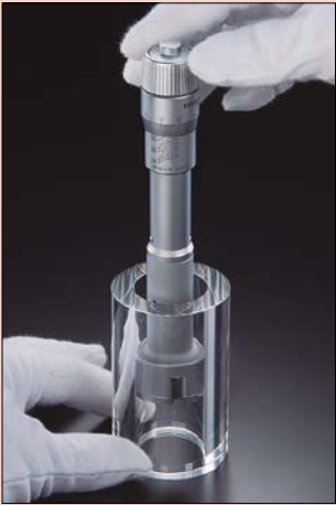
Constant-force device ensures repeatable measurement.
