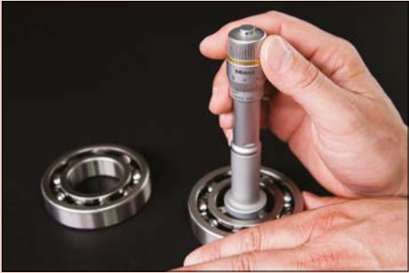
Ball-bearing inner-race inside diameter measurement.
