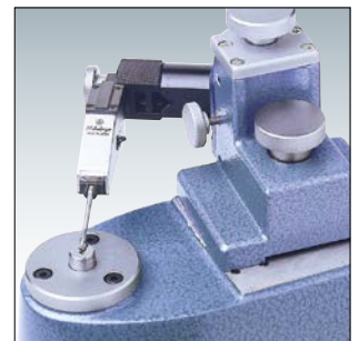
Calibrating a lever probe head.
