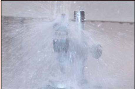
Rated to IP66 water- and dust-proofing standard and oil resistance improved.
