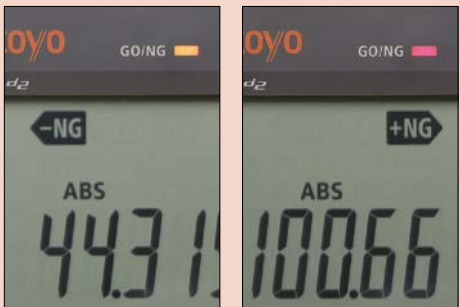
±NG shown on the display and the panel LED showing ORANGE (-NG) or RED (+NG) means the measurement is outside the tolerance limits.
