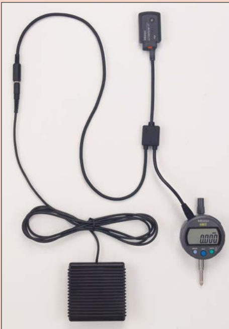
ABSOLUTE Digimatic Indicator ID-CX with 02AZD790F cable (footswitch optional accessory).
