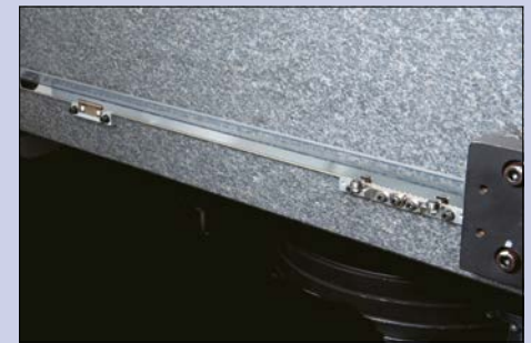
Dust-resistant high-precision glass scales.
