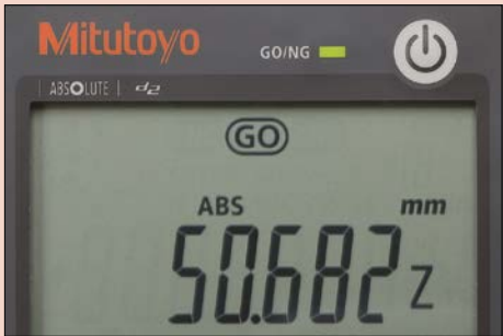
GO shown on the display and the panel LED showing GREEN means the measurement is within the tolerance limits.
