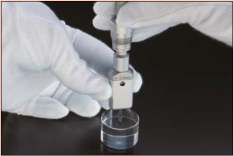
Measuring diameters down to 2 mm with the two-point model.
