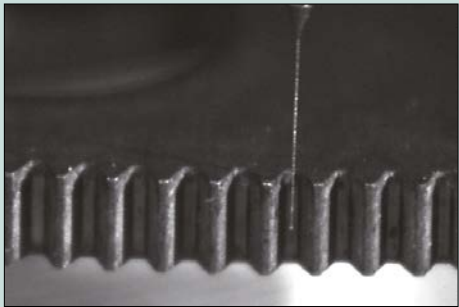
Measuring form accuracy of micro gear teeth.
