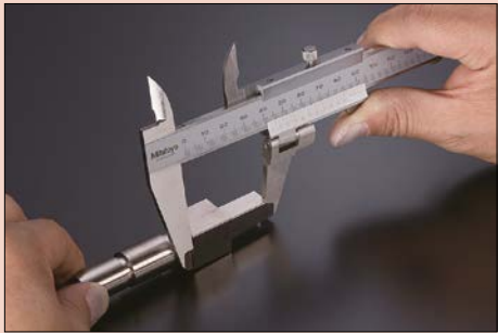
Measuring the distance from a shoulder to the end of a shaft.
