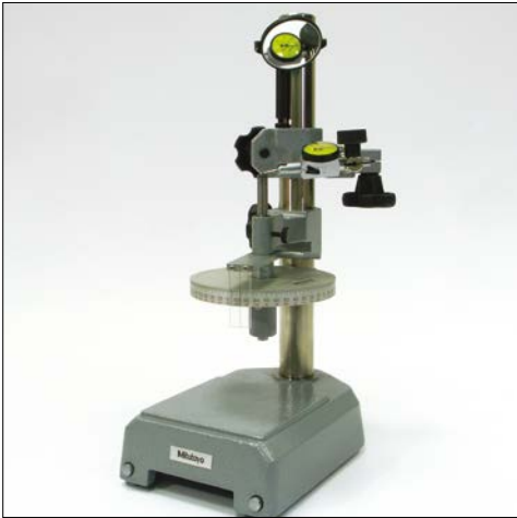
Calibrating a lever indicator.
