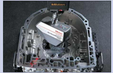
SurfaceMeasure probe scanning a complex surface.
