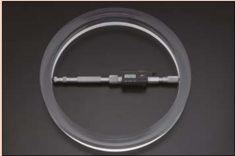
Using a setting ring to accurately set an inside micrometer.
