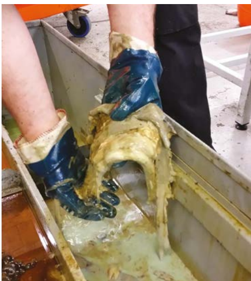
Figure 5: Biofilm deposits on the inside of MWF supply tank
