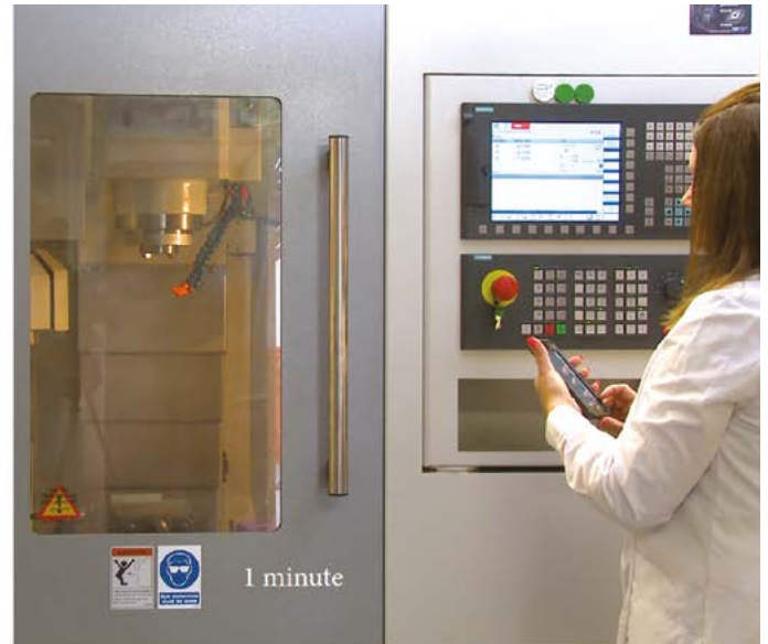
Figure 14b: Shows clearance of the smoke within a minute. Note, clearance times will differ depending on the size of the enclosure and the effectiveness of the LEV.
