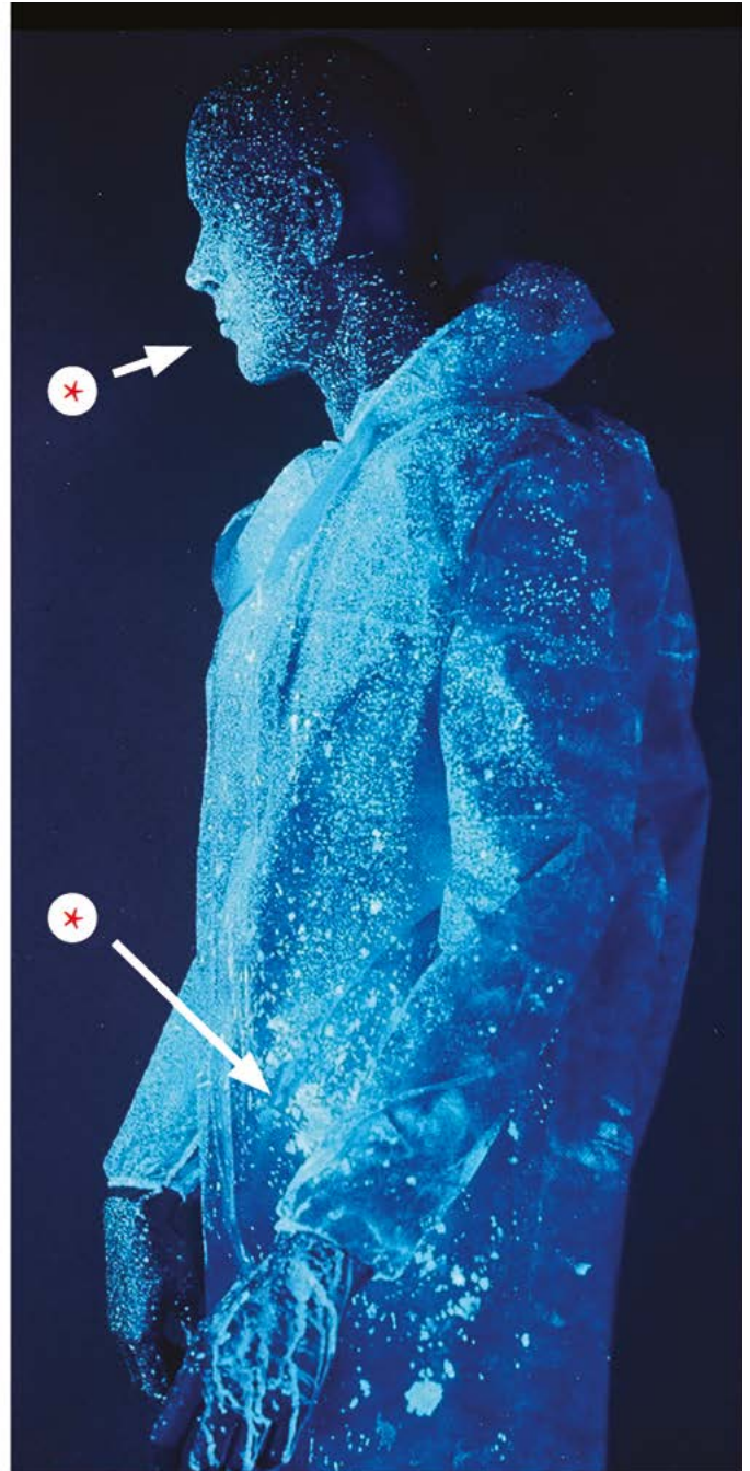
Figure 16: Shows a simulation of an operator using a compressed airline to remove MWF from a machined component, resulting in personal contamination with MWF droplets. The MWF was dosed with a blue dye, which under an ultra-violet lamp shows up as blue deposits on:
