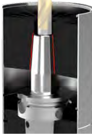
Bilz contact cooling system for air-cooled ISG machines
