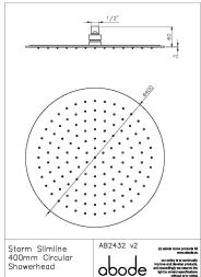
• Product mounted where: Roof / wall • Recommended hole size: N/A mm
