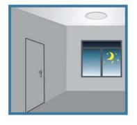
If with insufficient ambient light, the lamp dims to a stand-by dimming level (Set in the motion sensor) when no motion detected during hold time, and then switches off after stand-by period.
