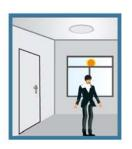
The lamp lights on 100% illumination or dims to maintain the preset illumination The lamp dims to level against ambient light.
