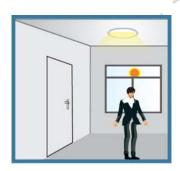
The lamp dims to minimum light level but never turn off even if with sufficient ambient light.
