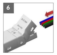
At the other end of the connecter, line up the wires so that the polarity matches the strip light.
