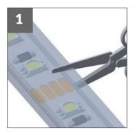
Cut strip light to the desired length using a sharp pair of scissors.
