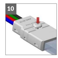
Place the stopper into the glue hole. Leave to dry for atleast 12 hours.
