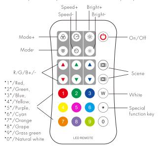
Mode+/-: Short press switch dynamic mode built in controller,
