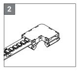
Insert the first LED strip into the longer side (21.8mm) of the corner connector.
