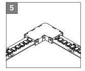
Close the buckles with a press. Make sure the connection is good with a small pull on the LED strip.
