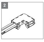
Insert the first LED strip into the longer side (19.7mm) of the corner connector.
