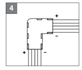
Check the polarity of the LED strip to make sure positive and negative line up.
