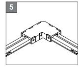
Close the buckles with a press. Make sure the connection is good with a small pull on the LED strip.
