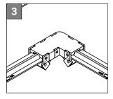
Insert the second LED strip into the corner connector.
