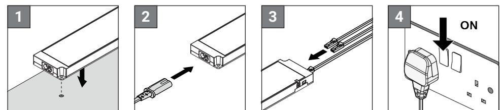
Mount the driver. Make sure it within 1.5 metres of a wall socket.
