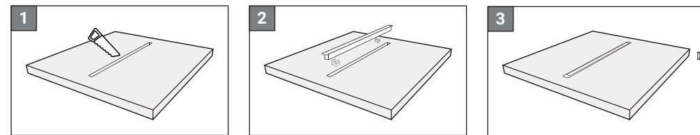
Make groove on the wooden shelf base in the Light bar size.
