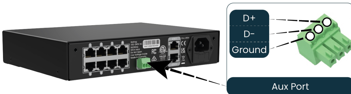
Figure 20: Location and Pinout of the Aux Port
