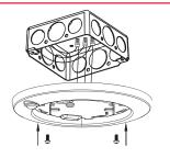
Align fixture and J Box 6 holes and attach fixture with provided screws. Do not over-tighten screws.
