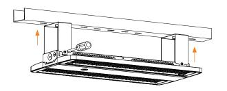
2 Assemble the fixture on the bracket and secure with screws.
