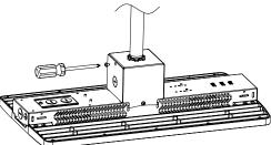
After wiring is secured within bracket mount, secure the side brackets onto the front and back of main bracket.
