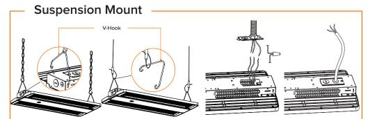
1 Attach chain or aircraft cable from ceiling to the fixture with the included V-Hooks. Adjust chain length as needed.
