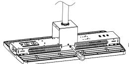
2 Lift the fixture to the bracket and secure the fixture. Connect the wires through the opening of the bracket.
