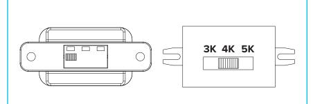
The fixture is Wattage and Kelvin Selectable. Adjustments can be made when the power is disabled.
