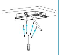
**↑** Disassemble the driver box by **↑** Loosen the 3/4" plug on the driver loosening the two screws on the driver housing.
