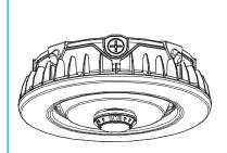
Disassemble the driver box by loosening the four screws on the driver housing with a screwdriver.
