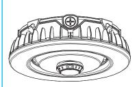
Disassemble the driver box by loosening the four screws on the driver housing with a screwdriver.
