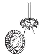
Attach the safety wire to the hook inside in the driver box.
