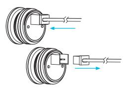
Photocell function is activated when connector is connected. Disconnection will deactivate the Photocell function.
