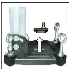
Remove the vacuum grip and the gasket of the base plate.
